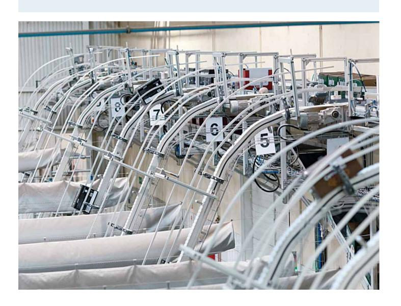
On traditional systems, large or bulky products require curves with a large radius and high friction coefficient. Rexroth takes a different approach: curves with ball bearings generate rolling friction. This means less friction and wear, as well as lower energy requirements and higher loads.
