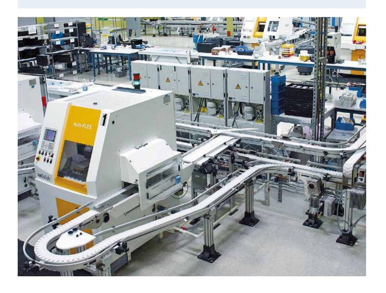
Even in nearly chip-free and modern machine tool linking, VarioFlow *plus* convinces with it use of largely mediaresistant components. Application in the lower load range is inexpensive and economic compared to previous, heavy systems.
