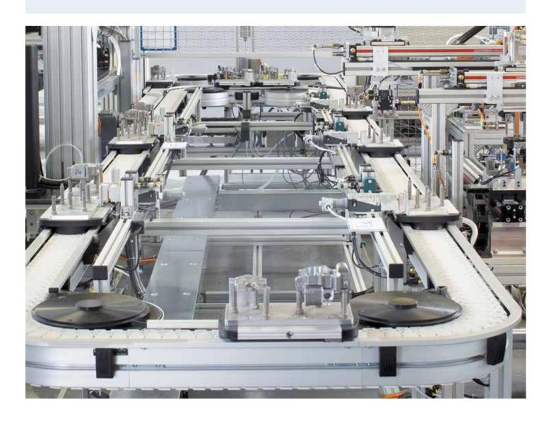
For parts transport between manufacturing processes – no matter whether semi or fully automatic stations or linked manual workplaces – the workpiece pallet conveyor system is the most effective solution. And it doesn't matter if the modular workpiece pallet system is provided by the customer or by Rexroth.
